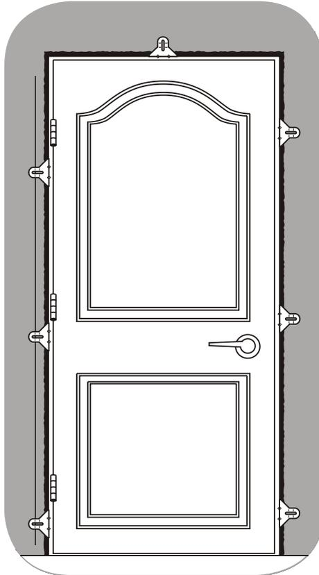
**NOTE:** For a premium installation, brackets may be used on both sides of an interior door. Add brackets to both the inside and outside of the door. Remove from the outside (non hinge side) and re-install as in exterior instructions.
